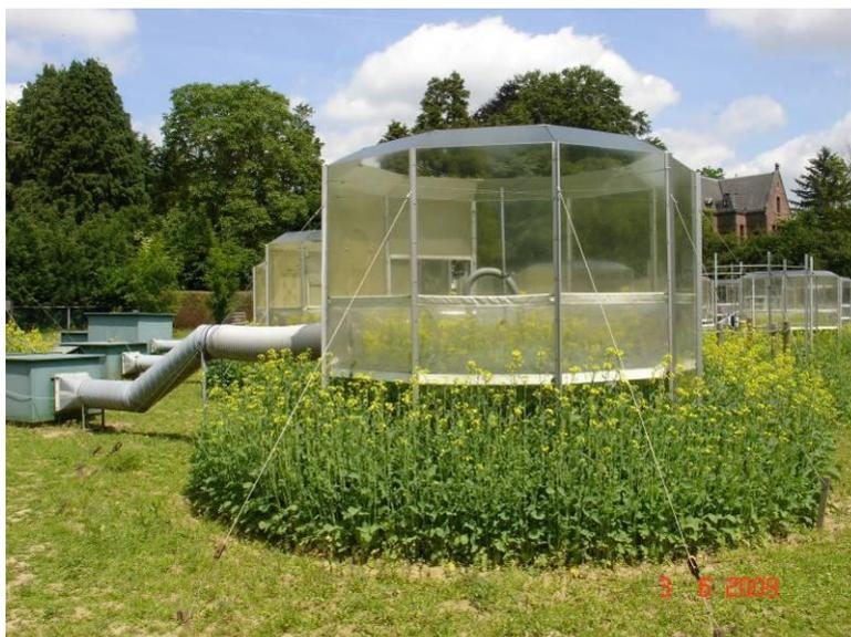
Figure 2: Open-Top Chambers for long term ozone exposure of oilseed rape and broccoli
