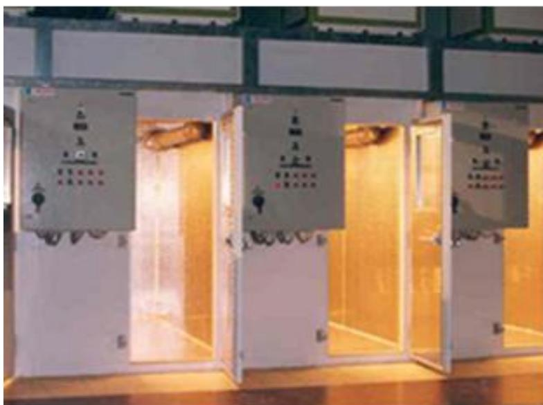
Figure 1: Environmentally controlled chambers for O<sub>3</sub> exposure
